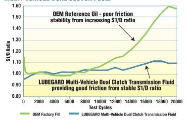
The S1/D measurement is commonly used to assess the overall friction quality between the lubricant and the clutch system. A stable S1/D ratio indicates good friction stability and an increasing S1/D ratio indicates poor friction stability.
